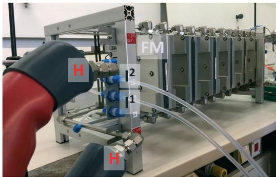
Fig. 7 Photograph of the Corning® Advanced Flow™ G1 SiC reactor. Key: H = inlet and outlet for the heat exchanging fluid; I<sup>1</sup> = inlet for DMC; I<sup>2</sup> = inlet for preheated glycerol and NBu<sub>4</sub>Br; FM = fluidic module.
