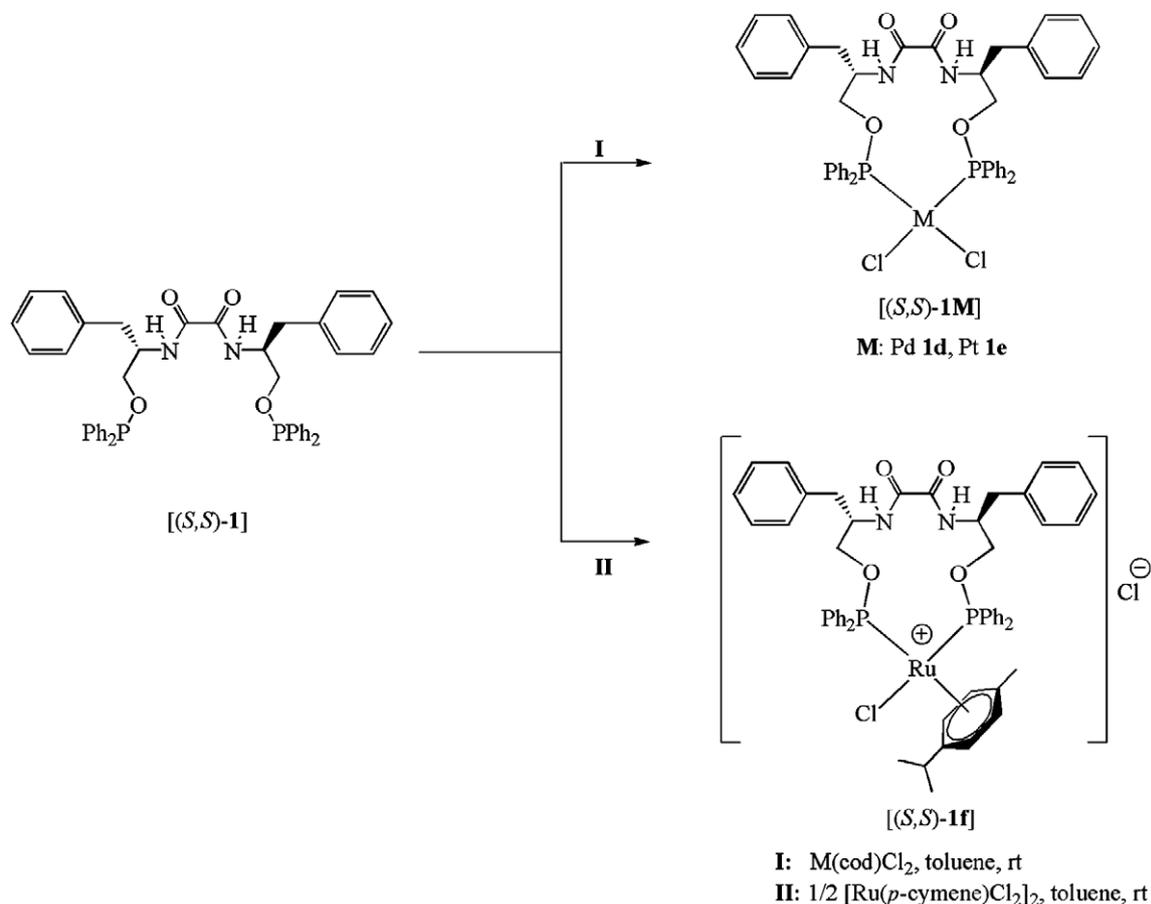
**Scheme 3.** Reactions of *N,N'*-bis[(1*S*)-1-benzyl-2-*O*-(diphenylphosphinite)ethyl]ethanediamide (**1**) with  $M(\text{cod})\text{Cl}_2$  ( $M$ : Pd (**1d**), Pt (**1e**)) and  $[\text{Ru}(p\text{-cymene})\text{Cl}_2]_2$  in toluene.
