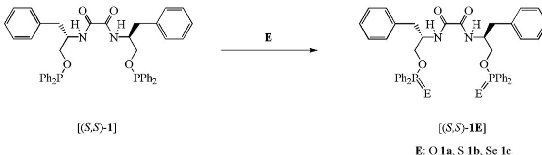
**Scheme 2.** Oxidation of  $N,N'$ -bis[(1*S*)-1-benzyl-2-*O*-(diphenylphosphinite)-ethyl]ethanediamide (**1**) with aqueous  $H_2O_2$  (**1a**), elemental sulfur (**1b**) and grey selenium (**1c**).
