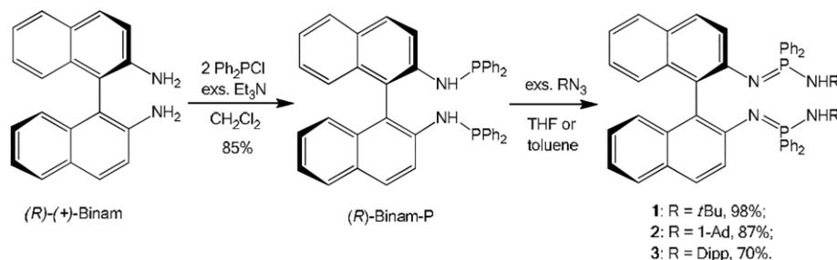
**Scheme 1.** Synthesis of (*R*)-Binam-P and therefrom derived bis-NPN ligands **1–3**.
