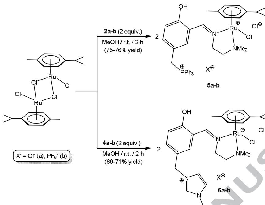
**Scheme 3.** Synthesis of arene-ruthenium(II) complexes **5-6a-b** containing an ionic Schiff-base ligand.
