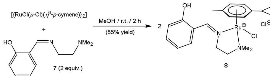
**Scheme 4.** Synthesis of the arene-ruthenium(II) complex **8** containing a neutral Schiff-base ligand.
