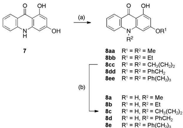
**Scheme 2.** Reagents: (a) alkyl halogenide, K<sub>2</sub>CO<sub>3</sub>, acetone, RT or reflux; (b) 48% HBr, reflux.
