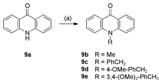
**Scheme 3.** Reagents: (a) alkyl halogenide, K<sub>2</sub>CO<sub>3</sub>, acetone, reflux.
