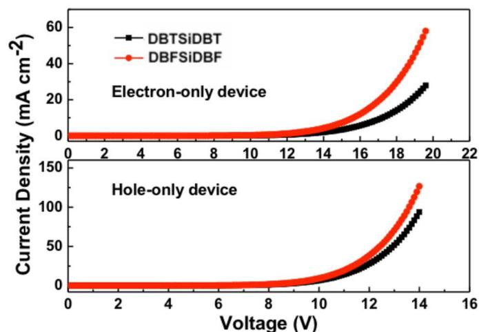
Figure 7.  $J$ - $V$  characteristics of hole- and electron-only devices. Hole-only devices: ITO/ MoO<sub>3</sub> (10 nm)/ **Host** (100 nm)/ MoO<sub>3</sub> (10 nm)/ Al (100 nm); electron-only devices: ITO/ TmPyPB (20 nm)/ **Host** (100 nm)/ TmPyPB (20 nm)/ Liq (2 nm)/ Al (100 nm).
