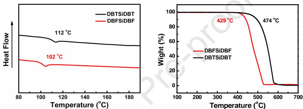
Figure 1. Differential scanning calorimetry (DSC, left) and thermogravimetric analyses (TGA, right) of **DBTSiDBT** and **DBFSiDBF**.
