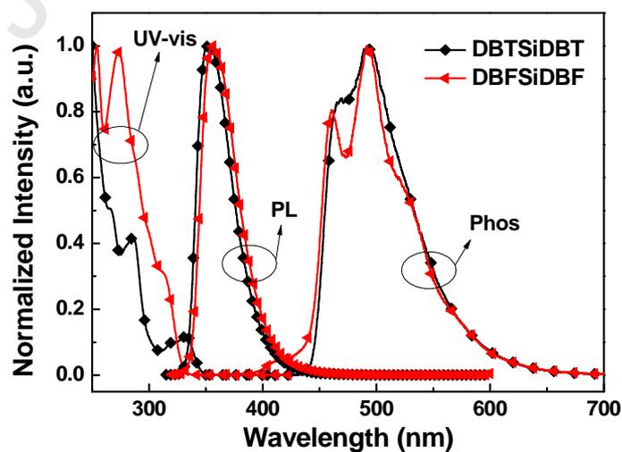
Figure 2. UV-Vis absorption, PL and Phos spectra of **DBTSiDBT** and **DBFSiDBF**.
