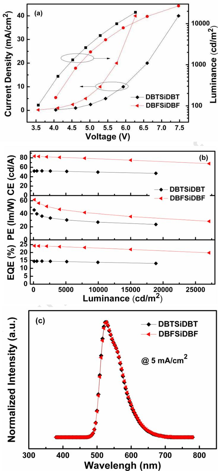
**Figure 6.** Current density–voltage–luminance ( $J$ - $V$ - $L$ ) characteristics (a); current efficiency (CE), Current density–voltage–luminance ( $J$ - $V$ - $L$ ) characteristics (a); current efficiency (CE), power efficiency (PE) and external quantum efficiency (EQE) versus luminance curves for Ir(ppy)<sub>3</sub>-based devices (b) and EL spectra at 5 mA/cm<sup>2</sup> (c).
