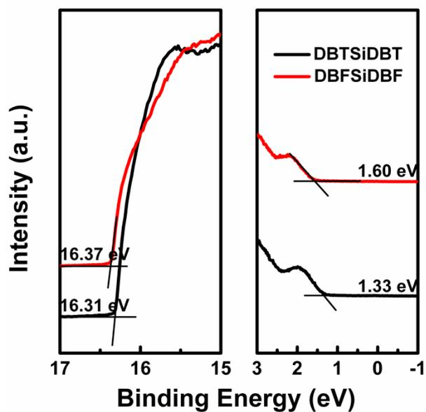
Figure 4. UPS spectra of DBTSiDBT and DBFSiDBF.
