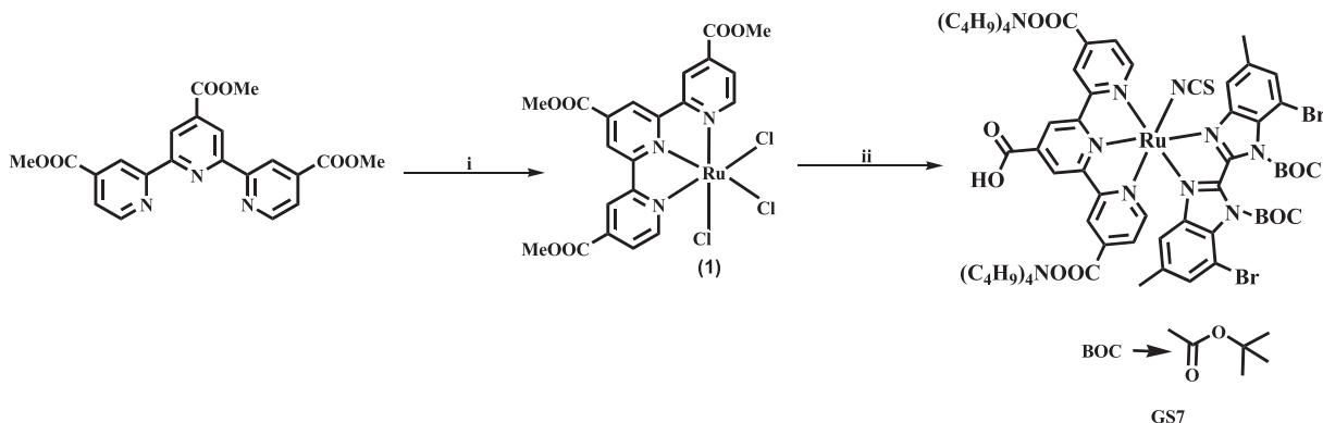
**Scheme 1.** Synthesis of sensitizer **GS7**. Reagents and conditions: i)  $\text{RuCl}_3 \cdot 3\text{H}_2\text{O}$ , anhydrous DMF, reflux under dark, 4 h; ii) L1, DMF reflux, 4 h then  $\text{NH}_4\text{NCS}$ , reflux, 2 h then TEA, water, reflux, 48 h.
