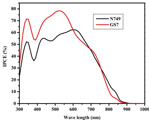
Fig. 5. IPCE spectra of **GS7** and N749 sensitizers.
