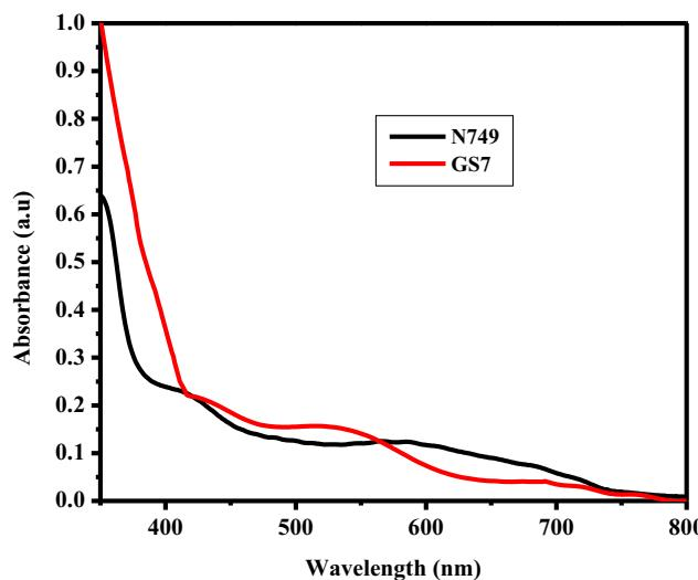
Fig. 3. Absorption spectra of **GS7** and N749 on  $\text{TiO}_2$ .
