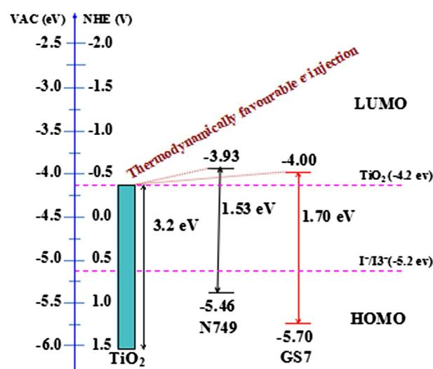
Fig. 4. Energy level diagram and comparison between HOMO and LUMO of **GS7** and N749.
