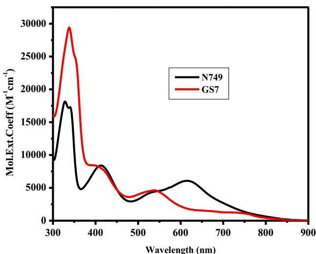
**Fig. 2.** Absorption spectra of **GS7** and N749 sensitizers in DMF.
