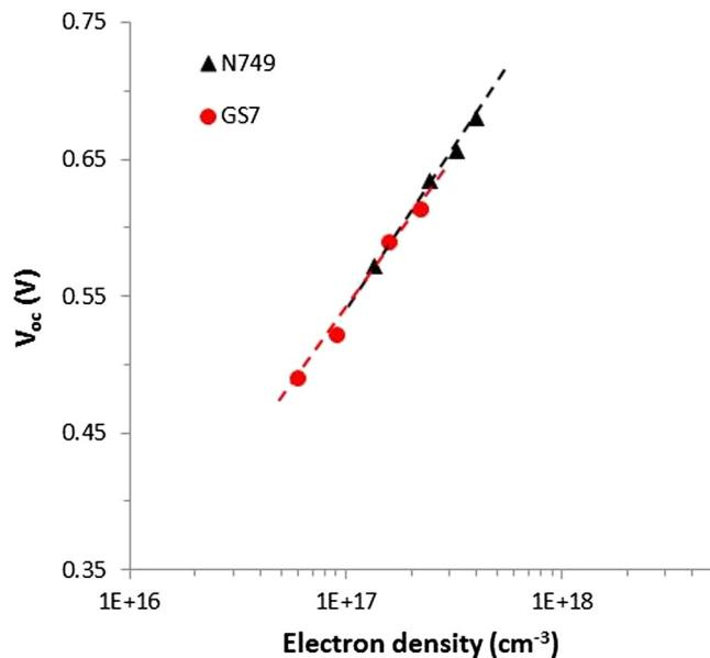
Fig. 7.  $V_{oc}$  as a function of electron density for DSSCs sensitized with N749 and **GS7**.
