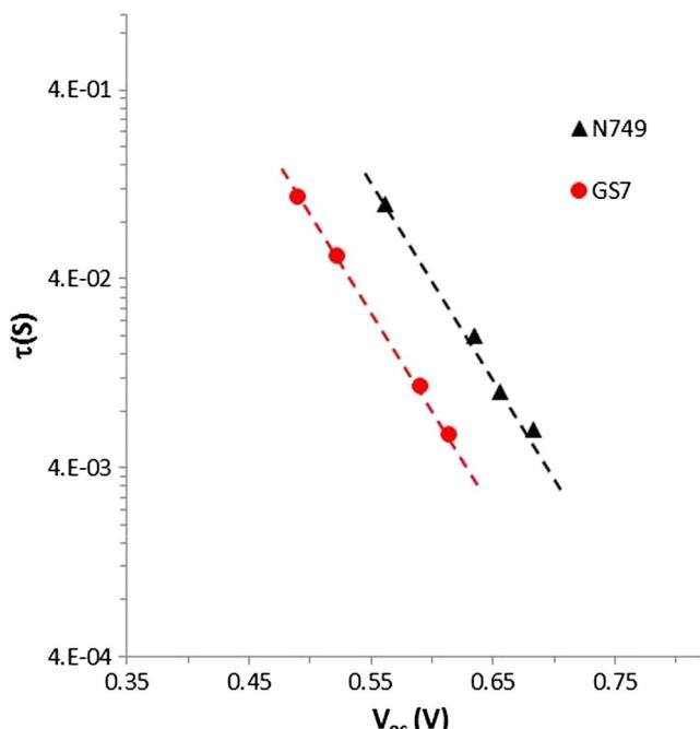
Fig. 8. Electron lifetime ( $\tau$ ) as a function of  $V_{oc}$  for DSSCs sensitized with N749 and **GS7**.
