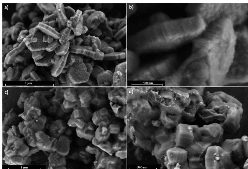
Fig. 1 HRSEM images of (a and b) calcined COK-12 and (c and d) TiO<sub>2</sub>-COK-12 platelets viewed at different magnifications.
