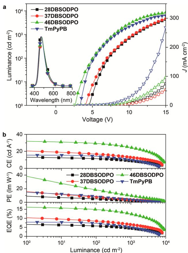
**Figure 7.** (a) Luminance–current density ( $J$ )–voltage characteristics and (b) efficiencies–luminance curves of *m*DBSODPO-based blue TADF devices in comparison to TmPyPB-based controls.
