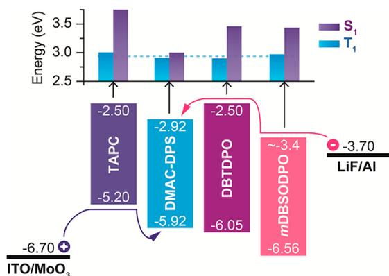
**Figure 6.** Device configuration of four-layer blue TADF devices and energy level diagram of FMOs and excited states of the employed materials.
