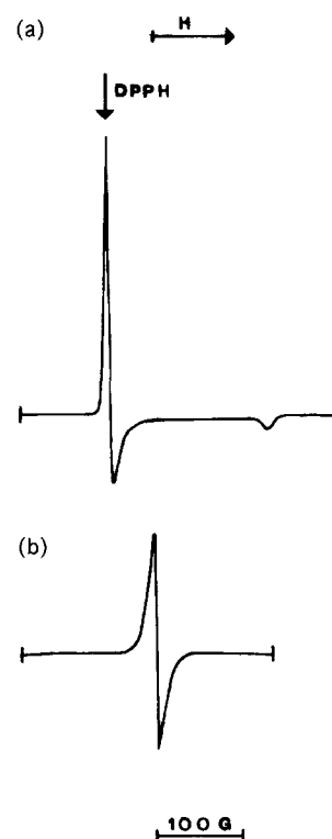
Fig. 2. X-band EPR spectra recorded at (a) 100 K and (b) 300 K on a THF solution of 4 after its first-stage electroreduction (about 0.5 electron per molecule) at 253 K.
