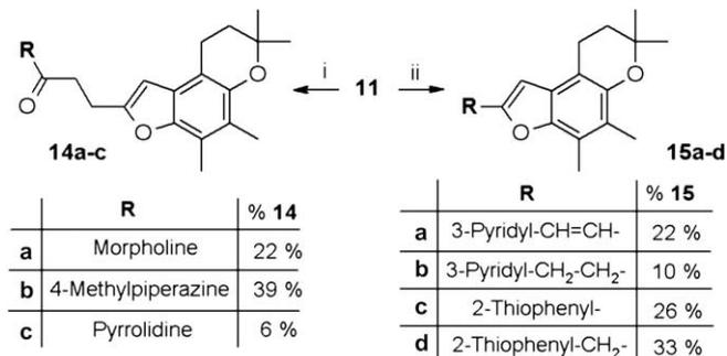
**Scheme 3.** (i) Succinic anhydride, amine, CH<sub>2</sub>Cl<sub>2</sub>, then DCC; 11, NEt<sub>3</sub>, heat. (ii) RCOOH, DCC, HOBT, (or RCOCl) NEt<sub>3</sub>, MeCN, 120 °C (microwave).
