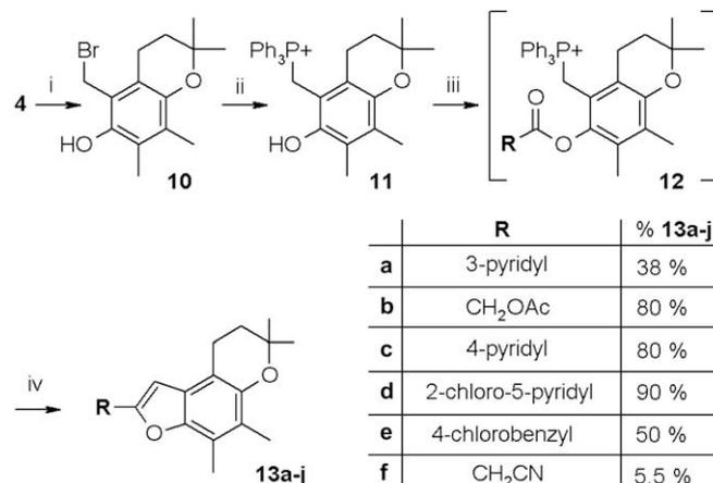
**Scheme 2.** (i) Br<sub>2</sub> cyclohexane. (ii) PPh<sub>3</sub>, CH<sub>2</sub>Cl<sub>2</sub> or cyclohexane. (iii) RCOCl or RCOOH, DCC, NEt<sub>3</sub>. (iv) NEt<sub>3</sub>, heat.
