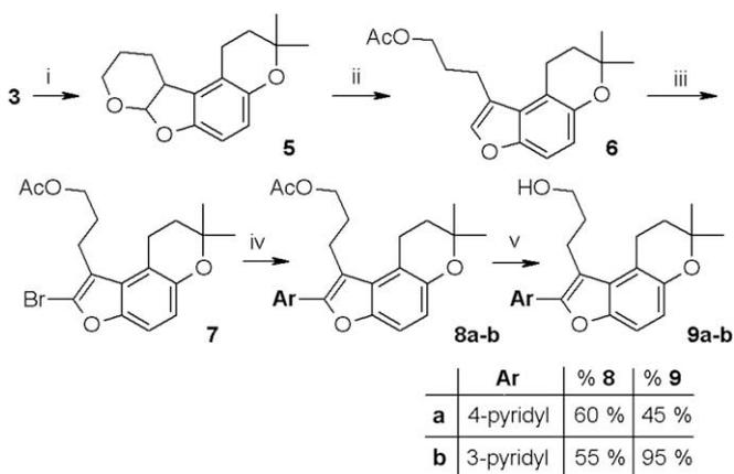
**Scheme 1.** (i) HCOOH, NH<sub>3</sub>, Pd/C ethanol reflux. (ii) AcOH, HCl reflux. (iii) NBS, EtOH. (iv) ArB(OH)<sub>2</sub>, Pd dppf, dioxane–water, Cs<sub>2</sub>CO<sub>3</sub>, 80 °C. (v) MeONa/MeOH.
