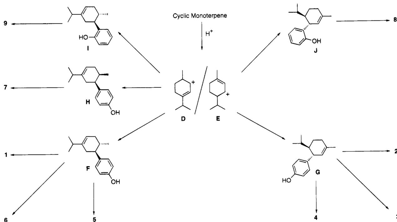
**Figure 4.** Mechanism of formation for products 1–9 from phenol and a cyclic monoterpene.
