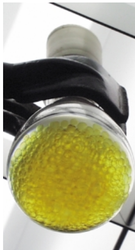
Figure 3. Round-bottomed flask containing a suspension of polymer beads p\text{-17}\cdot\text{AlMe} (diameter > 1000 \mu\text{m} ) in toluene.
