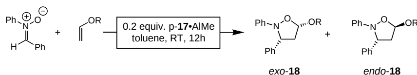
Scheme 11. 1,3-Dipolar cycloaddition of diphenyl nitron to vinyl ethers to give cycloadducts 18 , mediated by BINOL copolymers p\text{-17}\cdot\text{AlMe} . R = Et or t Bu.
