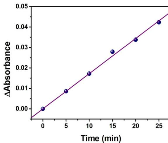
Fig. 3 A plot of the difference in absorbance ( $\Delta A$ ) vs time to evaluate the initial velocity of the catalytic oxidation of 3,5-DTBC by **1** in MeOH
