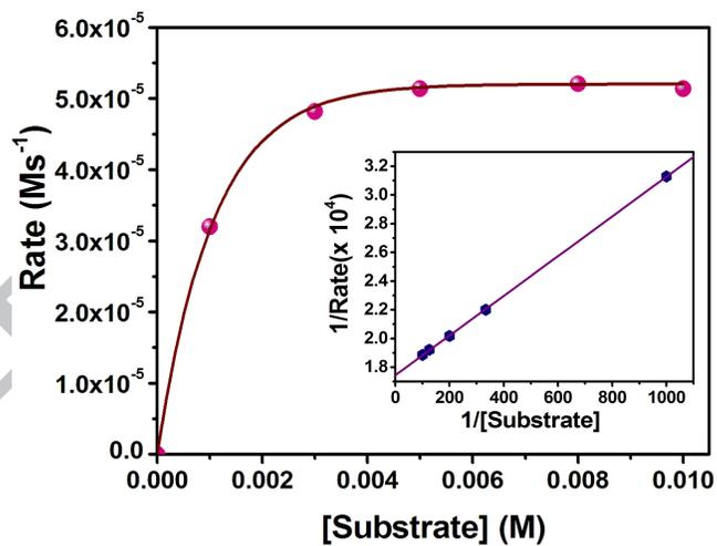
Fig. 4 Plot of rate vs. [substrate] in the presence of **1** in MeOH; inset: Lineweaver-Burk plot
