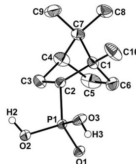
Figure 4. Structure of *endo*-bornylphosphonic acid (**6a**) showing 30% probability displacement ellipsoids and the numbering scheme.
