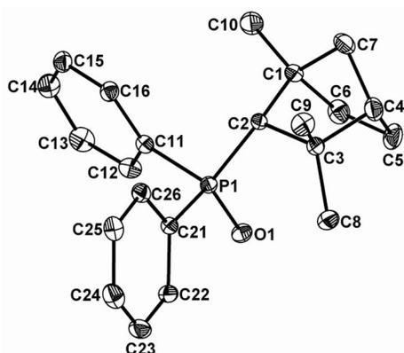
Figure 2. Structure of *endo*- $\alpha$ -fenchyldiphenylphosphane oxide (**8a**) showing 30% probability displacement ellipsoids and the numbering scheme.
