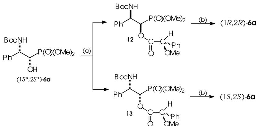
Scheme 5. Reagents and conditions: (a) (*S*)-Ph(MeO)CHCOOH, DCC, DMAP, (b) aqueous NH<sub>3</sub>, THF
