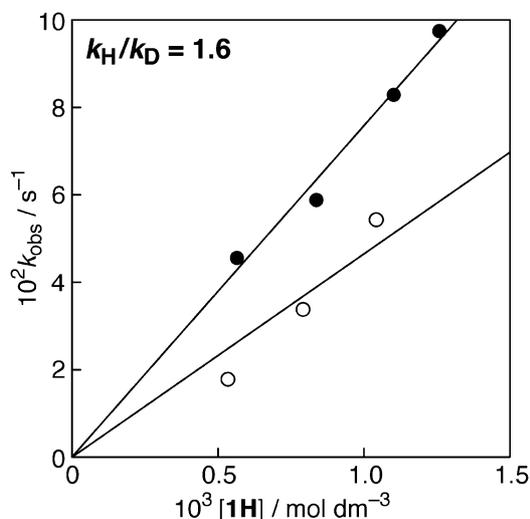
**Figure 5.** Plots of  $k_{\text{obs}}$  vs.  $[\mathbf{1H}]$  in the presence of  $\text{CH}_3\text{OH}$  ( $3.5 \times 10^{-1} \text{ mol dm}^{-3}$ ) (closed circles) and  $\text{CD}_3\text{OD}$  ( $3.5 \times 10^{-1} \text{ mol dm}^{-3}$ ) (open circles) for the reaction between **1H** and  $\text{DPPH}^*$  ( $6.6 \times 10^{-5} \text{ mol dm}^{-3}$ ) in deaerated MeCN at 298 K.
