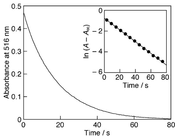
**Figure 1.** Time course of the absorbance change at 516 nm in the reaction of **7H** ( $2.0 \times 10^{-3} \text{ mol dm}^{-3}$ ) with DPPH' ( $4.0 \times 10^{-5} \text{ mol dm}^{-3}$ ) in deaerated MeCN at 298 K. Inset: The pseudo-first-order plot.
