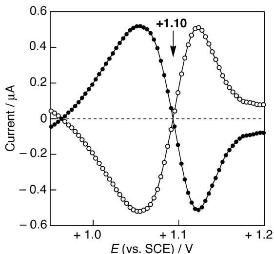
**Figure 4.** Second-harmonic alternating current voltammogram for the one-electron oxidation of **4H** ( $1.0 \times 10^{-3} \text{ mol dm}^{-3}$ ) in deaerated MeCN ( $0.1 \text{ mol dm}^{-3} \text{ Bu}_4\text{NClO}_4$ ) at 298 K. Scan rate:  $4 \text{ mV s}^{-1}$ ; amplitude:  $25 \text{ mV}$ .
