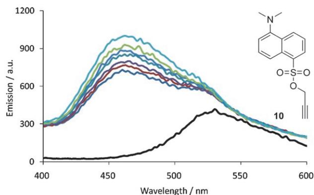
Figure 4. Fluorescence data of the inclusion of **10** in the CD cavities of the polymersomes.  $\lambda_{\text{exc}} = 305$  nm, emission range 400–600 nm. Black line: emission of free **10** in water (40  $\mu\text{M}$ ). Other traces: emission of the suspension of the polymersomes after adding different aliquots (from 1 to 10  $\mu\text{L}$ ) of **10**.
