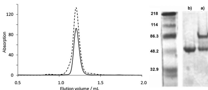
Figure 6. Left: FPLC of HRP (—) and HRP modified with compound **15** (----) at  $\lambda = 403$  nm. Right: SDS-PAGE of a) HRP modified with compound **15** after dialysis; b) HRP native (non-modified).
