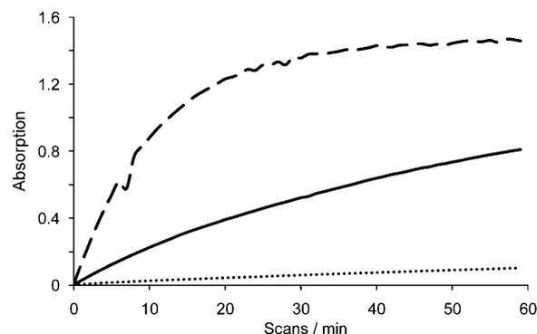
Figure 7. Activity measurements of HRP-PEG at  $\lambda = 420$  nm: blank eluate after 17 rinsing steps (.....); experimental eluate after 17 rinsing steps (---); activity retained in polymersomes after 25 rinsing steps (—).
