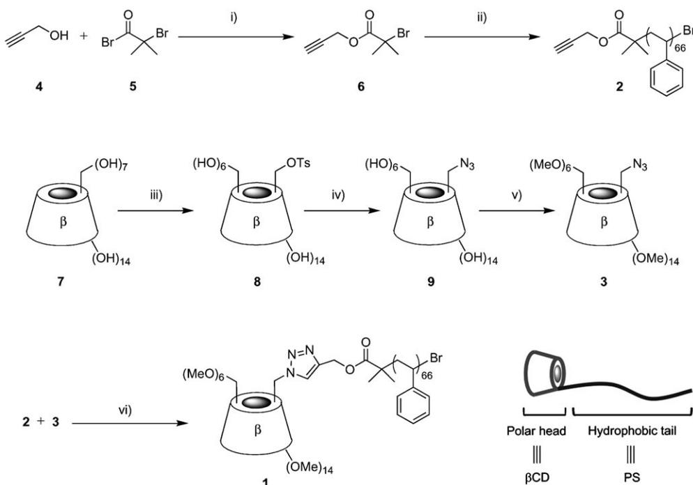
Scheme 2. Preparation of **1** and its precursors **2** and **3**. Bottom right: schematic representation of **1**. Reagents and conditions: i) diethyl ether, pyridine,  $-30^{\circ}\text{C} \rightarrow \text{RT}$ ; ii) CuBr, PMDTA, anisole,  $90^{\circ}\text{C}$ ; iii) NaOH, TsCl,  $\text{H}_2\text{O}$ ; iv)  $\text{NaN}_3$ , DMF,  $60^{\circ}\text{C}$ ; v) DMF, NaH,  $\text{CH}_3\text{I}$ ; vi) CuBr, PMDTA, THF under  $\text{N}_2$ .
