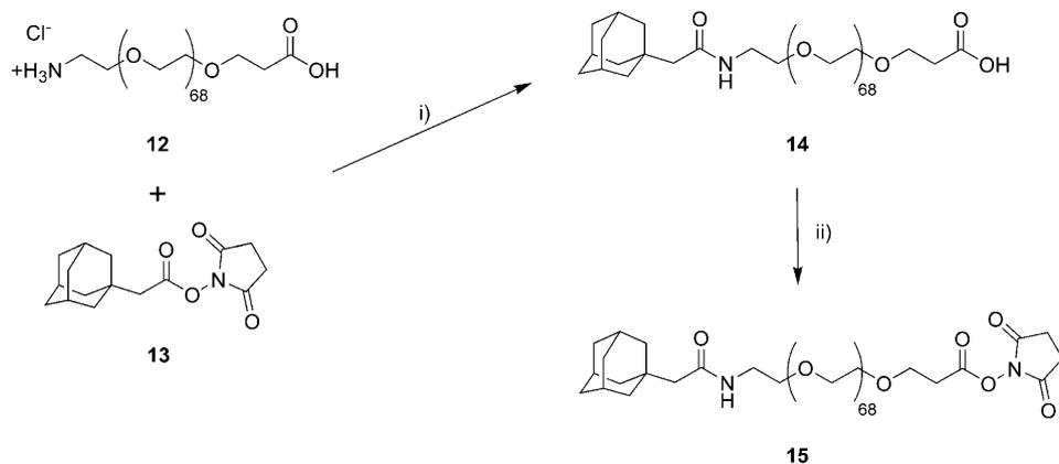
Scheme 3. Synthesis of adamantyl compound **15**. Reagents and conditions: i)  $\text{Et}_3\text{N}$ , dichloromethane; ii) *N*-hydroxysuccinimide, *N*-(3-dimethylaminopropyl)-*N*-ethylcarbodiimide (EDCI),  $\text{CH}_2\text{Cl}_2$ , from 0 °C to RT.
