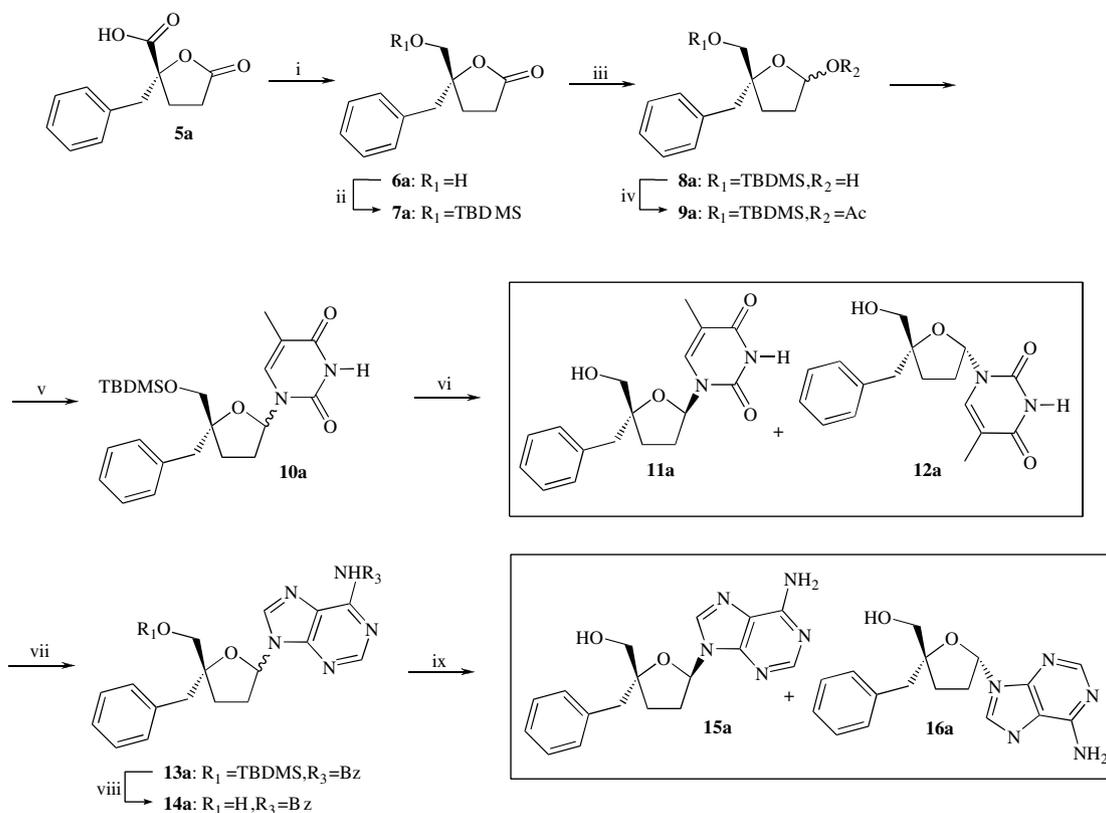
**Scheme 3.** Synthesis of 4'-benzyl substituted nucleoside analogues. Reagents: (i) BH<sub>3</sub>·SMe<sub>2</sub>/THF; (ii) TBDMSCl, imidazole/CH<sub>2</sub>Cl<sub>2</sub>; (iii) DIBAH/toluene, (iv) Ac<sub>2</sub>O/Et<sub>3</sub>N/CH<sub>2</sub>Cl<sub>2</sub>; (v) Thymine, BSA, TMSOTf/CH<sub>3</sub>CN; (vi) TBAF/THF; (vii) *N*<sup>6</sup>-benzoyladenine, BSA, TMSOTf/CH<sub>3</sub>CN; (viii) TBAF/THF; (ix) NH<sub>3</sub>/MeOH.
