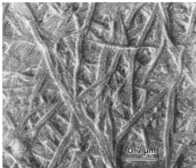
Figure 9. Freeze-fracture electron micrograph of a 1.85% (w/w) CAB in hexadecane gel; etched at -40 °C and 10 -7 Torr for 1 h.
