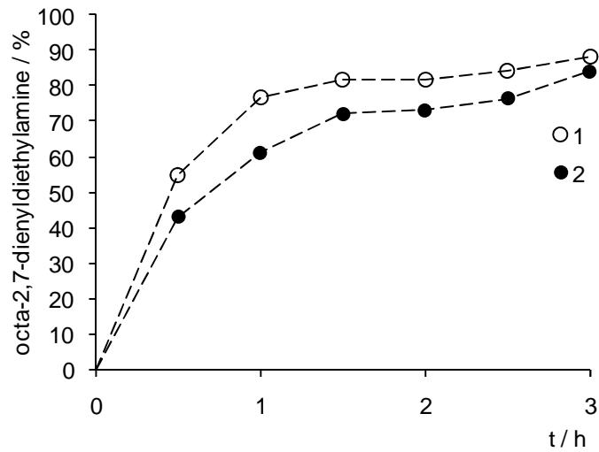
**Figure 3.** Activity, expressed as yields of octa-2,7-dienyldiethylamine as a function of reaction time. (Complex **5** was formed *in situ* by reaction of **8** with 2PPh<sub>3</sub> in dichloromethane. Reaction conditions: (1) BD:Pd = 6000, Et<sub>2</sub>NH:Pd = 3000, 1.3·10<sup>-5</sup> mol Pd, 70°C, 3 h, 0.5 ml CH<sub>2</sub>Cl<sub>2</sub> (2) BD:Pd = 3000, Et<sub>2</sub>NH:Pd = 6000, 0.65·10<sup>-5</sup> mol Pd, 70°C, 3 h, 0.5 ml CH<sub>2</sub>Cl<sub>2</sub>)
