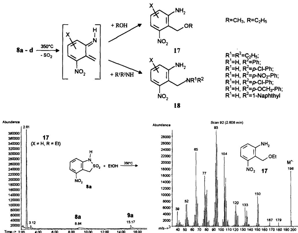
**Figure 2.** Injection of the solution of **8a** in ethanol at 350°C. Gas chromatogram (left) and mass spectrum (right) of the adduct **17** (X = H, R = Et).
