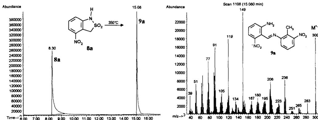
Figure 1. Injection of **8a** at 350°C. Gas chromatogram (left) and mass spectrum of the dimer **9a** (right).
