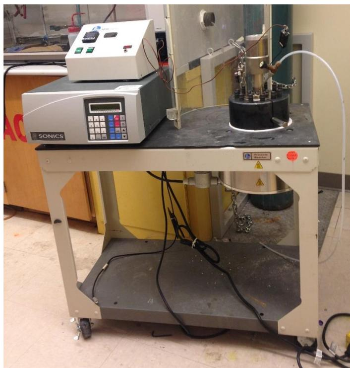
Figure S1 Parr temperature controller model 4838
