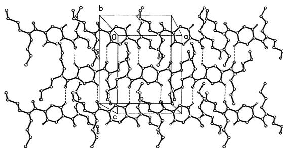
Fig. 11. Packing diagram for **4**. Hydrogen atoms not involved in hydrogen bonding are omitted. Hydrogen bonds are indicated by dashed lines. Radii are arbitrary.
