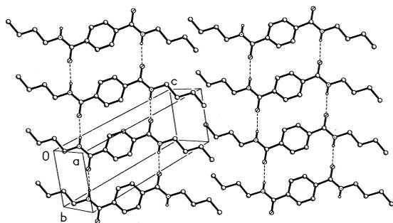
Fig. 8. Packing diagram for **1**. Hydrogen atoms not involved in hydrogen bonding are omitted. Hydrogen bonds are indicated by dashed lines. Radii are arbitrary.
