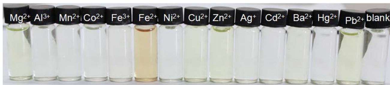
Fig. 3 Color change of compound L (10 \mu\text{M} ) in the presence of metal ions in EtOH–H 2 O mixed solvent
