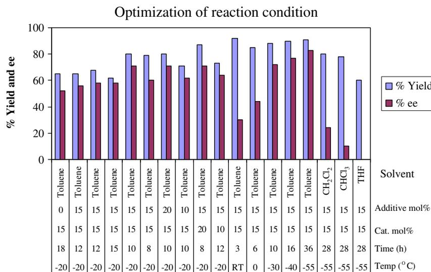
**Figure 2.** Optimization graph for the enantioselective addition of TMSCN to 4-MeO *N*-benzyl imines (**e**) using the catalyst **1**.
