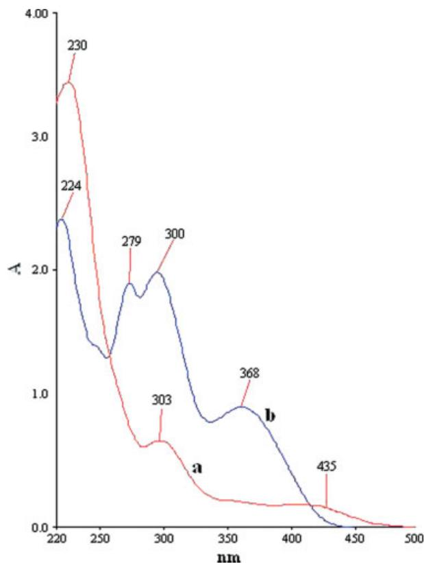
**Figure 1.** The UV-vis spectra of  $[\text{LBPh}_2]$  **2** (a) and  $[\text{LBF}_2]$  **3** (b) dissolved in  $\text{C}_2\text{H}_5\text{OH}$  at room temperature.
