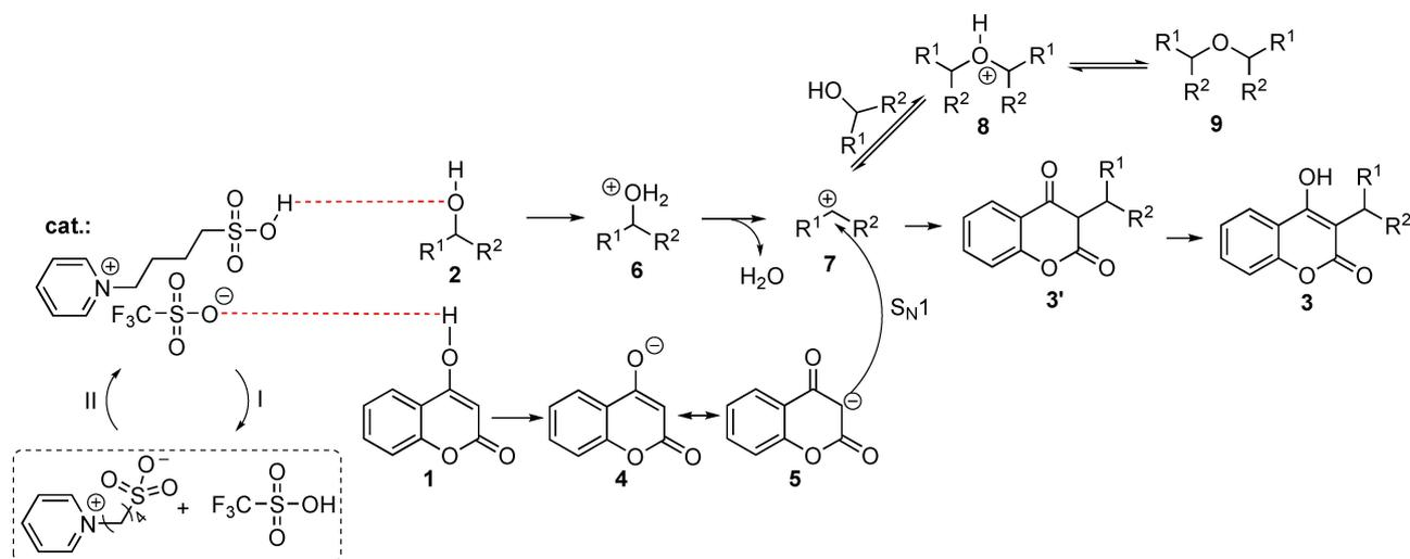
Scheme 6. Proposed mechanism for the substitution under the reaction conditions.
