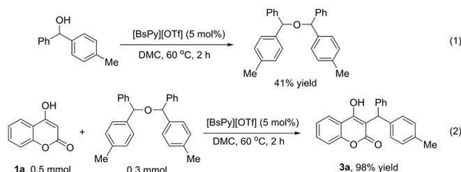
Scheme 5. Control experiments for the substitution of 4-hydroxycoumarin with phenyl(*p*-tolyl)methanol.
