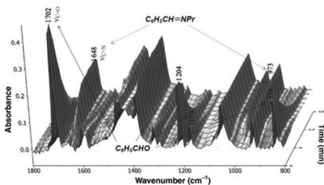
FIGURE 2 A segment of the time-dependent IR spectrum for the reaction of benzaldehyde with *n*-propylamine in acetonitrile at 0°C.
