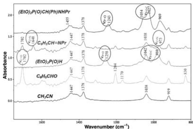
FIGURE 1 IR spectra of the reaction components measured in acetonitrile solution.
