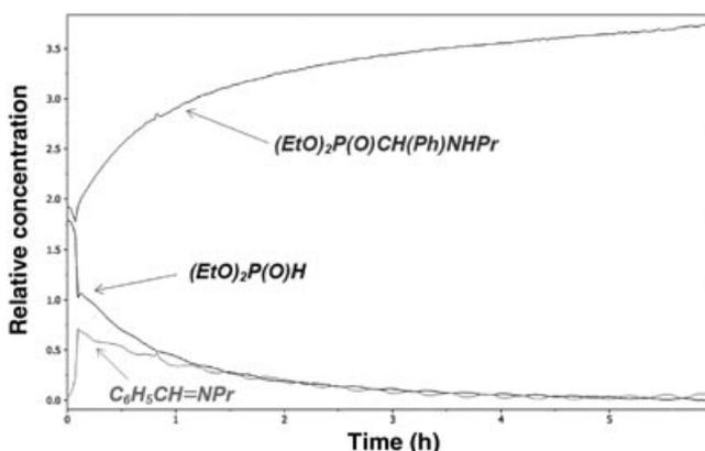
FIGURE 7 Concentration profile for the Kabachnik–Fields reaction studied at 80°C in acetonitrile.
