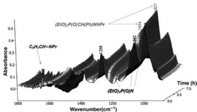
FIGURE 6 A segment of the time-dependent IR spectrum for the Kabachnik–Fields reaction of diethyl phosphite, *n*-propylamine, and benzaldehyde at 80°C in acetonitrile.
