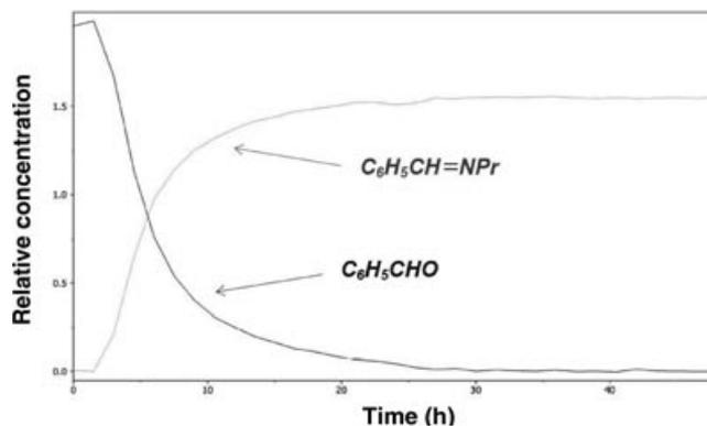
FIGURE 3 Concentration profile for the reaction of benzaldehyde with *n*-propylamine at 0°C in acetonitrile.
