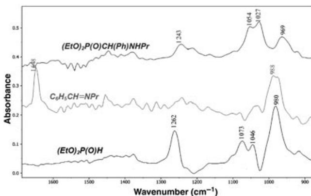
FIGURE 8 IR spectra for the reaction components obtained from the 3D diagram after deconvolution.
