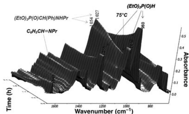
FIGURE 4 A segment of the time-dependent IR spectrum for the reaction of imine **1** with diethyl phosphite in acetonitrile.
