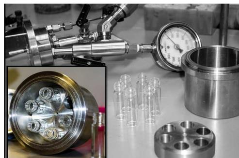
**Figure 2.** Parallelized hydrogenation setup in Parr<sup>TM</sup> pressure reactors.
