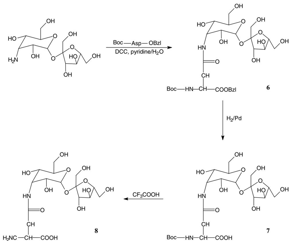
**Figure 1.** Synthesis of 3-(*N-tert*-butoxycarbonyl-L-aspartic acid-4-amido-1-benzyl ester)-3-deoxy- $\alpha$ -D-allopyranosyl  $\beta$ -D-fructofuranoside (**6**), 3-(*N-tert*-butoxycarbonyl-L-aspartic acid 4-amido)-3-deoxy- $\alpha$ -D-allopyranosyl  $\beta$ -D-fructofuranoside (**7**), and 3-(L-aspartic acid 4-amido)-3-deoxy- $\alpha$ -D-allopyranosyl  $\beta$ -D-fructofuranoside (**8**).
