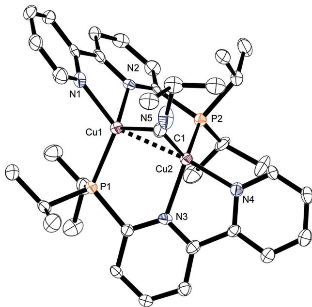
Figure 4. Molecular structure of **4**. The counterions, hydrogen atoms, and co-crystallized solvent molecules have been omitted for clarity. Thermal ellipsoids are shown at 50% probability. Selected bond lengths [Å] and angles [°]: Cu1–Cu2 2.5124(9), Cu1–N1 2.053(4), Cu1–C1 2.054(6), Cu1–N2 2.089(4); N1–Cu1–C1 103.8(2), N1–Cu1–N2 78.73(17), C1–Cu1–N2 113.05(19), N1–Cu1–P1 122.02(13), C1–Cu1–P1 118.69(16), N2–Cu1–P1 113.95(13).
