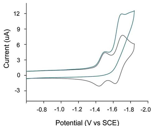
Figure 6. Cyclic voltammogram of [Cu<sub>2</sub>(μ-PPh<sub>2</sub>-Me<sub>2</sub>-bipy)<sub>2</sub>(NCCH<sub>3</sub>)<sub>2</sub>](PF<sub>6</sub>)<sub>2</sub> (**1**) under N<sub>2</sub> and under CO<sub>2</sub> in acetonitrile with 0.1 M TBAH.
