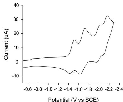
Figure 5. Cyclic voltammogram of [Cu<sub>2</sub>(μ-PPh<sub>2</sub>-Me<sub>2</sub>-bipy)<sub>2</sub>(NCCH<sub>3</sub>)<sub>2</sub>](PF<sub>6</sub>)<sub>2</sub> (**1**) under N<sub>2</sub> in acetonitrile with 0.1 M TBAH.
