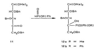
These results showed that the reaction of glycosuloses and other ketones with phosphonates and phosphinates having a P-H bond gives 1:1 adducts in good yields; hence, the reaction seems to provide a good method for preparing sugar derivatives containing a phosphorus-carbon bond. The stereospecificity and reaction rate of addition of phosphorus compounds were controlled mainly by substituents adjacent to the carbonyl group, as well as by the conformation (steric-approach control<sup>15</sup>).
