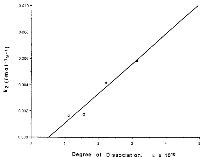
Figure 5. Acree plot for the alkylation of sodium phenolate with methyl iodide in tetrahydrofuran at 25 °C.
