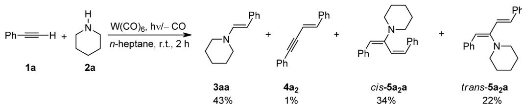
**Scheme 2.** Reaction of phenylacetylene **1a** and piperidine **2a** in the presence of photochemically activated W(CO)<sub>6</sub> **1b**.
