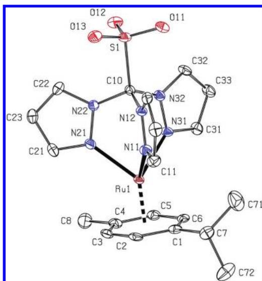
**Figure 3.** ORTEP diagram of the  $[\text{Ru}(p\text{-cymene})(\text{Tpms})]^+$  cation in **4**, with atomic numbering scheme. Ellipsoids are drawn at 50% probability. Hydrogen atoms and  $\text{BF}_4^-$  counterion are omitted for clarity. Selected bond distances (Å) and angles (deg): N11–Ru1 2.101(2), N21–Ru1 2.092(2), N31–Ru1 2.082(2), N11–N12 1.372(3), N21–N22 1.374(3), N31–N32 1.362(3), C10–S1 1.894(3); N21–Ru1–N11 79.34(9), N31–Ru1–N11 83.03(8), N31–Ru1–N21 84.44(9).
