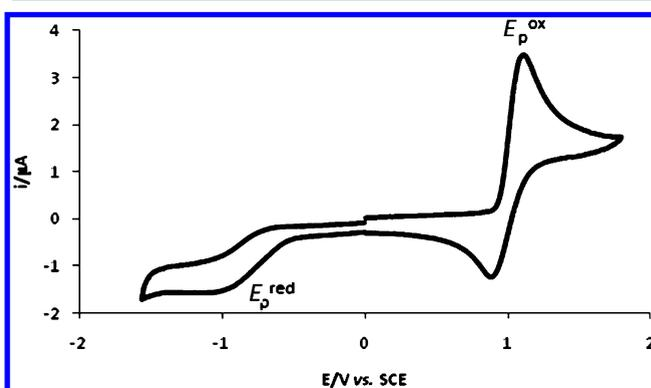
**Figure 4.** Cyclic voltammogram of [Ru(*p*-cymene)(Tpms)]BF<sub>4</sub> (4), in a 0.2 M [<sup>n</sup>Bu<sub>4</sub>N][BF<sub>4</sub>]/NcMe solution, at a Pt disk working electrode ( $d = 0.5$  mm), run at a scan rate of 200 mV s<sup>-1</sup>, starting with the anodic sweep (potential in V vs SCE).
