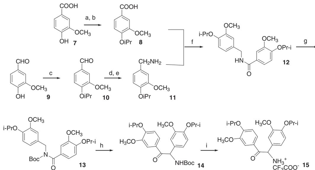
**Scheme 2.** Reagents and conditions: (a) *i*PrBr,  $K_2CO_3$ , DMF, reflux, 4 h, 98%; (b) KOH, ethanol,  $H_2O$ , reflux, 4 h, 86%; (c) *i*PrBr,  $Na_2CO_3$ , DMF, reflux, 4 h, 91%; (d)  $NH_2OH \cdot HCl$ , Py, ethanol, rt, 90 min, 71%; (e) Ni/Al alloy, NaOH 2 N, ethanol, rt, 90 min, 98%; (f) HOBt, WSC, THF, rt, 24 h, 96%; (g) *di-tert*-butyldicarbonate, DMAP, acetonitrile, rt, 16 h, 95%; (h) LDA, DMPU, THF,  $-78^\circ C$ , 8 h, 55%; (i)  $CF_3COOH$ , DCM, rt, 2 h, 98%.
