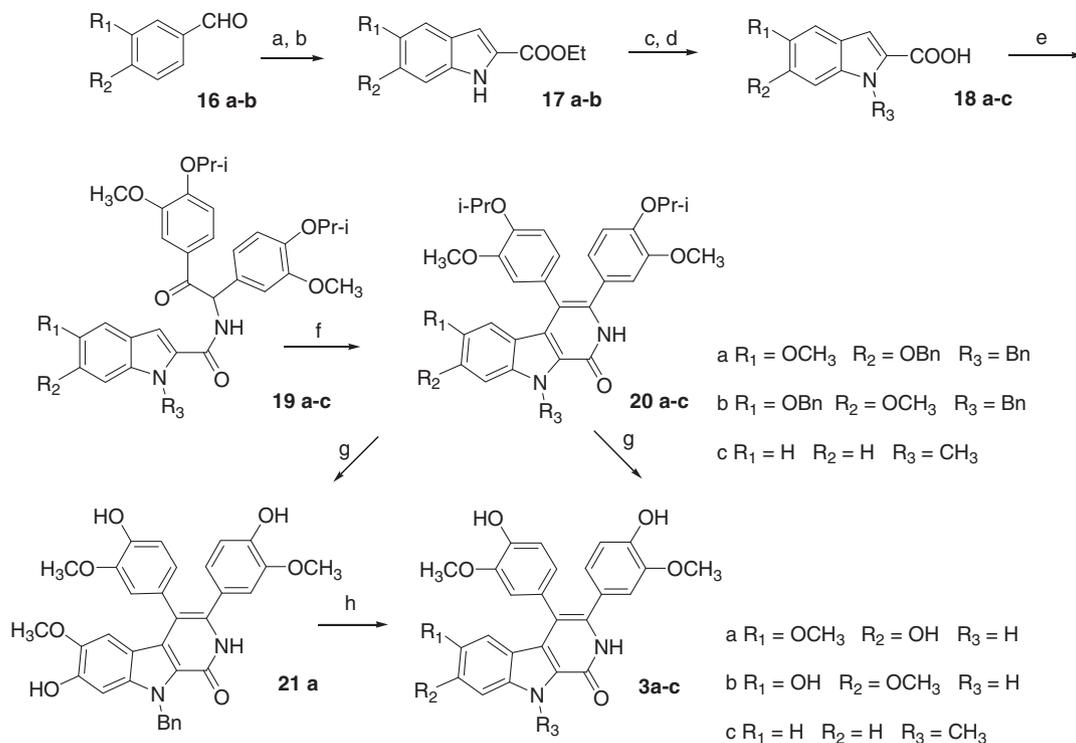
**Scheme 3.** Reagents and conditions: (a) ethyl azidoacetate, EtONa, EtOH, -15 °C, 3 h, 73–88%; (b) xylene, reflux, 12 h, 32–76%; (c) for **17a–b**: BnBr, NaH, DMF, 0 °C–rt, 2 h, 67–97%; (d) LiOH, H<sub>2</sub>O, THF, MeOH, rt, 4 h, 64–76%; (e) HOBt (1-hydroxybenzotriazole), WSC, **15**, TEA, THF, rt, 14 h, 56–58%; (f) TFA, acetonitrile, reflux, 15 min, 58–71%; (g) AlCl<sub>3</sub>, DCM, 0 °C–rt, 24 h, 30–48%; (h) for **3a**: AlCl<sub>3</sub>, anisole, 100 °C, 5 h, 20%.
