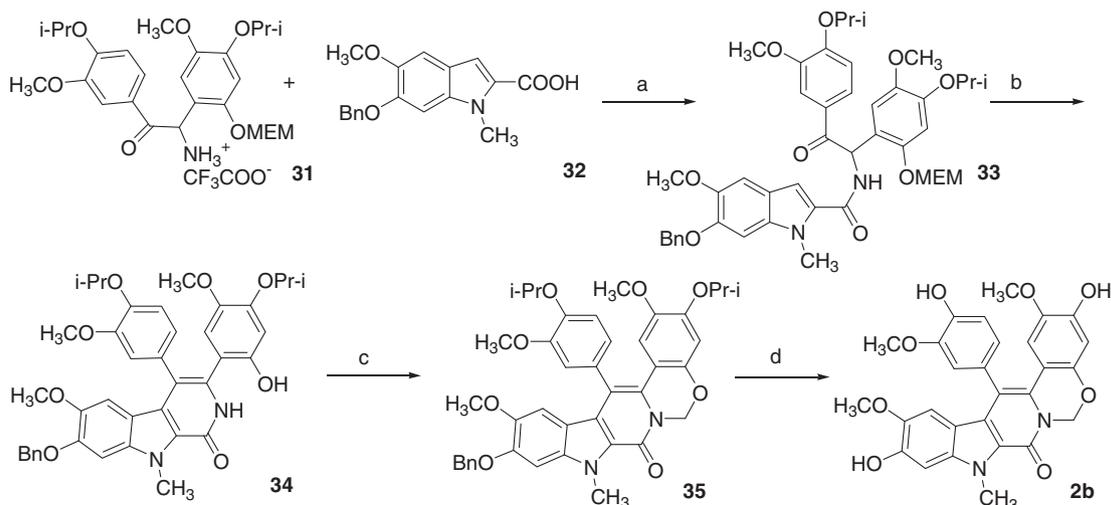
**Scheme 5.** Reagents and conditions: (a) HOBt, WSC, TEA, THF, rt, 26 h, 55%; (b) NaI, TMSI, acetonitrile, –20 °C, 30 min, 31%; (c) CH<sub>2</sub>I<sub>2</sub>, DCM, reflux, 1 h, 12%; (d) AlCl<sub>3</sub>, DCM, reflux, 6 h, 83%.
