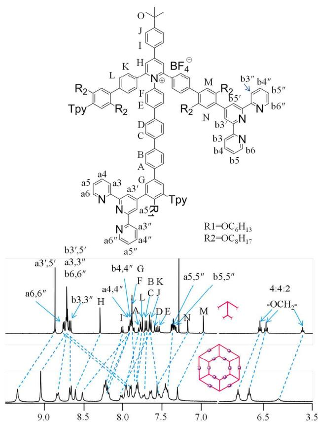
**Figure 6.** <sup>1</sup>H NMR spectra (400 MHz) of ligand LD in CDCl<sub>3</sub> and complex [Zn<sub>12</sub>LD<sub>6</sub>] in CD<sub>3</sub>CN. "Tpy" was used to replace the terpyridine structure.
