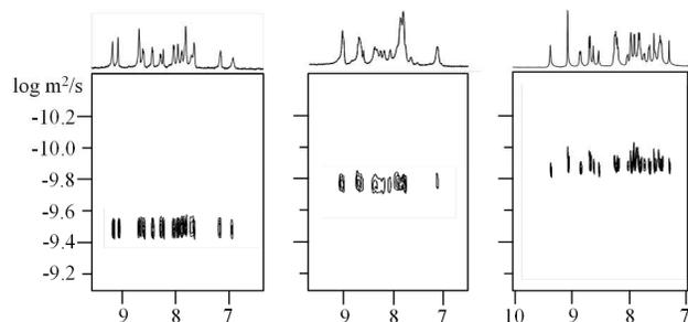
**Figure 9.** 2D DOSY NMR spectra of  $[\text{Zn}_{12}\text{LB}_6]$  (left),  $[\text{Zn}_{12}\text{LC}_6]$  (middle), and  $[\text{Zn}_{12}\text{LD}_6]$  (right) (500 Hz,  $\text{CD}_3\text{CN}$ , 300 K).
