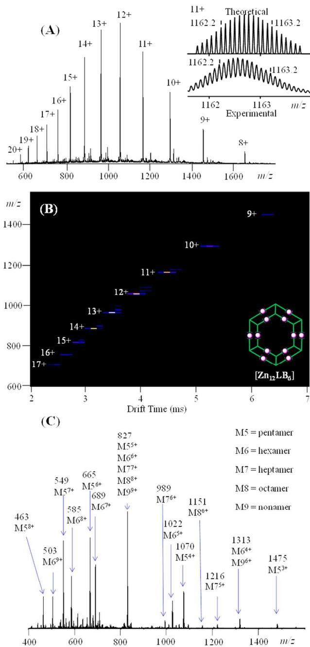
**Figure 3.** (A) ESI-MS and (B) 2D ESI-TWIM-MS plot ( $m/z$  vs. drift time) of complex  $[\text{Zn}_{12}\text{LB}_6]$ . (C) ESI-MS of multiple macrocycles assembled by ditopic ligand **5** with  $\text{Zn}(\text{II})$ .
