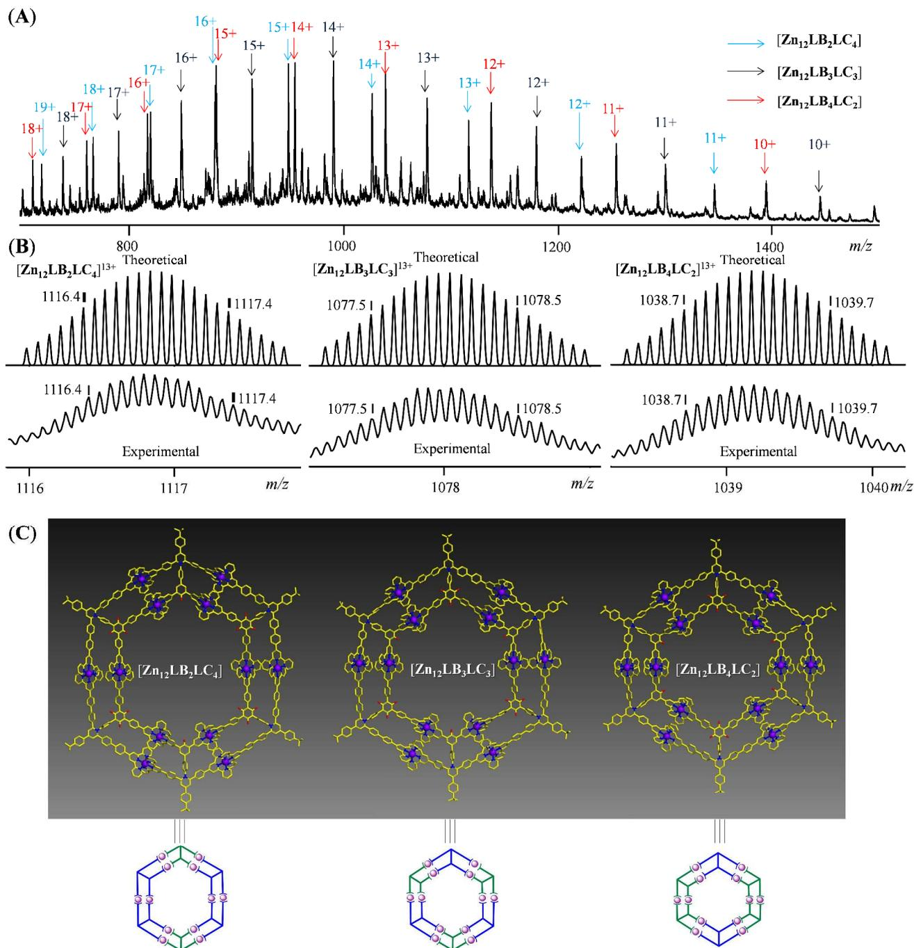
**Figure 8.** (A) ESI-MS of mixture of hybrid concentric hexagons. (B) The theoretical and experimental isotopic patterns of the 13+ signals. (C) Energy-minimized structures of  $[\text{Zn}_{12}\text{LB}_2\text{LC}_4]$ ,  $[\text{Zn}_{12}\text{LB}_3\text{LC}_3]$  and  $[\text{Zn}_{12}\text{LB}_4\text{LC}_2]$ . The alkyl chains are omitted for clarity in the molecular modeling.
