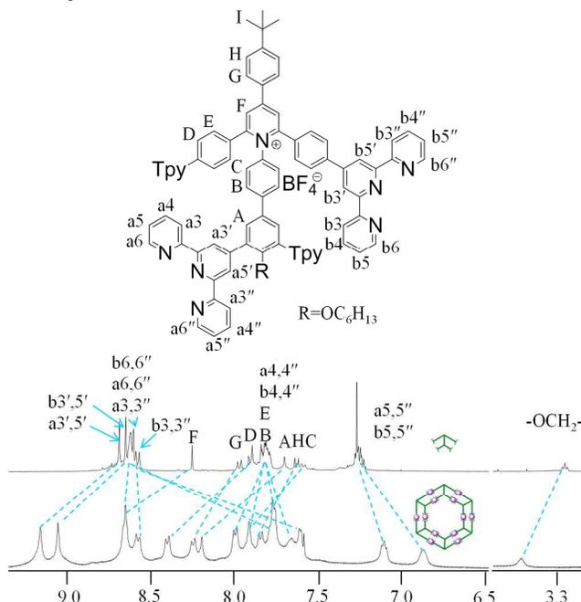
**Figure 2.** <sup>1</sup>H NMR spectra (400 MHz) of ligand **LB** in  $\text{CDCl}_3$  and complex  $[\text{Zn}_{12}\text{LB}_6]$  in  $\text{CD}_3\text{CN}$ . "Tpy" was used to replace the terpyridine structure.
