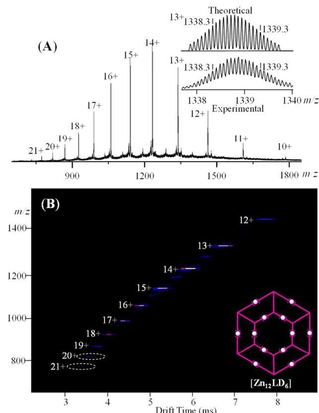
**Figure 7.** (A) ESI-MS and (B) 2D ESI-TWIM-MS plot (*m/z* vs. drift time) of complex [Zn<sub>12</sub>LD<sub>6</sub>]. The charge states of intact assemblies are marked.
