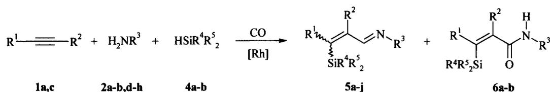
Scheme 4. Silylformylation of acetylenes in the presence of primary amines
