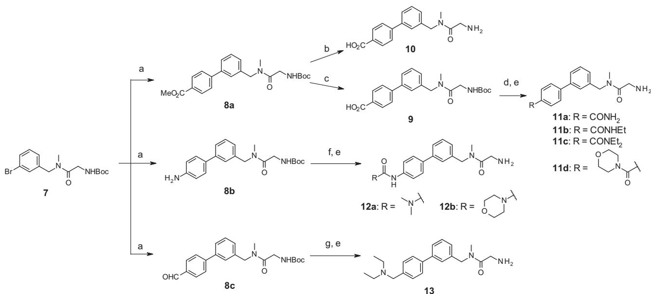
**Scheme 3.** Reagents and conditions: (a) Ar-B(OH)<sub>2</sub> or Ar-B(Pin), Pd(PPh<sub>3</sub>)<sub>4</sub>, Na<sub>2</sub>CO<sub>3</sub>, DME/EtOH/H<sub>2</sub>O, 80 °C; (b) 6 M HCl aq, 100 °C; (c) 1 M NaOH aq, MeOH; (d) amine, WSCD-HCl or WSCD, HOBt, with or without Et<sub>3</sub>N, DMF; (e) 4 M HCl (EtOAc solution), solvents; (f) carbamoyl chloride, base, CH<sub>2</sub>Cl<sub>2</sub>; (g) diethylamine, NaBH(OAc)<sub>3</sub>, AcOH, DCE.
