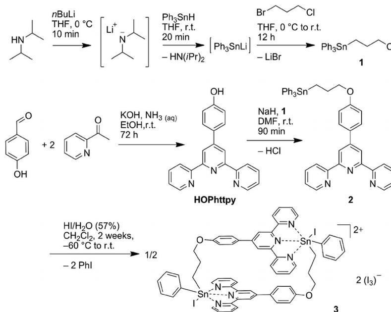
Scheme 2. Synthesis pathway for the terpyridine functionalized tinorganyl **2** with an overall yield of 51%, and subsequent reaction to form the dinuclear complex cation within compound **3**.
