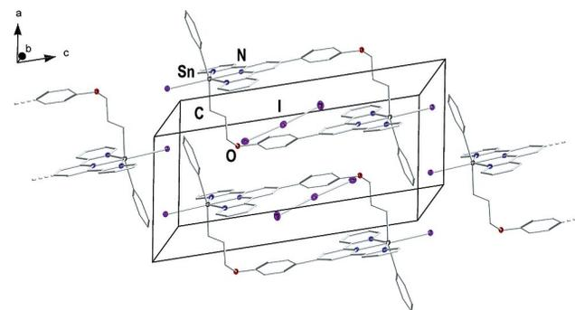
Figure 4. Arrangement of the molecules in the crystal structure of **3**. H atoms are omitted for clarity. C atoms are denoted as sticks. Thermal ellipsoids are drawn at 50% probability.
