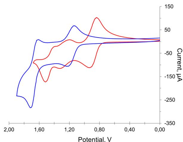
**Figure 4.** Cyclic voltammograms of [(PhPy)Pd( $\mu$ -OAc)] (**1**; red) and [(PhPy)Pd( $\mu$ -TFA)]<sub>2</sub> (**2**; blue) in  $\text{CH}_2\text{Cl}_2$ .
