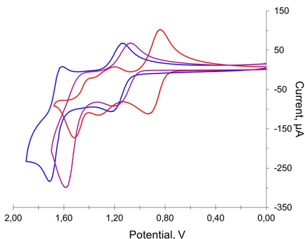
**Figure 7.** Cyclic voltammograms of  $[(\text{PhPy})\text{Pd}(\mu\text{-OAc})]_2$  in the absence (red) and in the presence (6 equiv) of  $\text{H}(\text{CF}_2)_4\text{COOH}$  (violet) in  $\text{CH}_2\text{Cl}_2$  in comparison with  $[(\text{PhPy})\text{Pd}(\mu\text{-TFA})]_2$  (blue).
