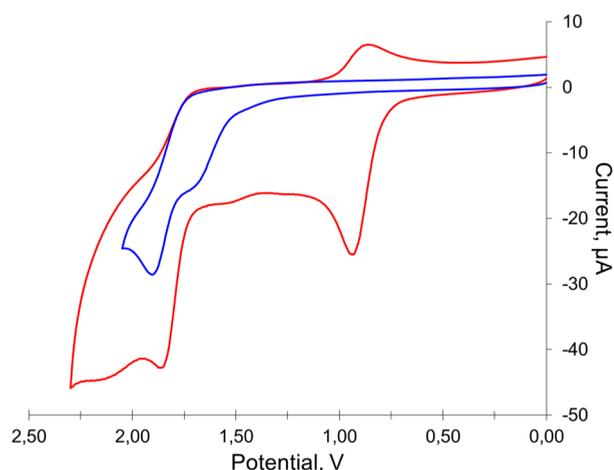
**Figure 5.** Cyclic voltammograms of [(PhPy)Pd( $\mu$ -OAc)]<sub>2</sub> (**1**; red) and [(PhPy)Pd(TFA)]( $\text{CH}_3\text{CN}$ ) (**3**; blue) in  $\text{CH}_3\text{CN}$ .
