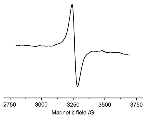
**Figure 6.** ESR spectrum obtained upon oxidation of [(PhPy)Pd(μ-OAc)]<sub>2</sub> (**1**) (CH<sub>2</sub>Cl<sub>2</sub> solution, room temperature, 0.9 V vs Ag/AgCl).
