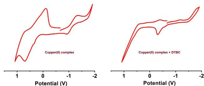
**Fig. 4.** Left: Cyclic voltammogram of the copper(II) complex **1** in  $\text{CH}_2\text{Cl}_2$ ; Right: Cyclic voltammogram of copper(II) complex **1** in presence of DTBC under molecular oxygen atmosphere in  $\text{CH}_2\text{Cl}_2$ .
