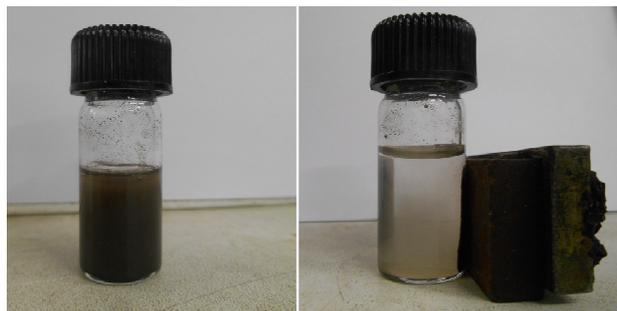
**Fig: 9** Magnetic recoverability of catalyst by external magnet
