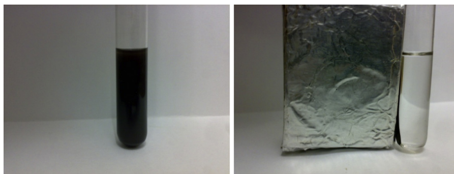
Fig. 5. Image showing MNPs-Guanidine can be separated by applied magnetic field. A reaction mixture in the absence (left) or presence of a magnetic field (right).
