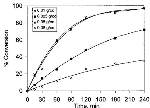
**Figure 3.** Effect of catalyst loading on benzene alkylation with 1-dodecene. C<sub>12</sub>:C<sub>6</sub>H<sub>6</sub>, 1:10 mol; catalyst DTP/K-10, 0.05 g/mL, temperature, 150 °C; speed, 1000 rpm; reaction time, 4 h.
