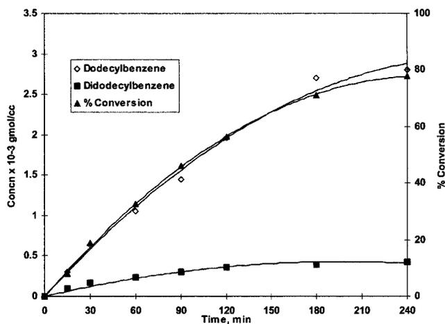
**Figure 5.** Effect of mol ratio on yields of mono- and dialkylated products in benzene alkylation with 1-dodecene. C<sub>12</sub>:C<sub>6</sub>H<sub>6</sub>, 1:2 mol; catalyst DTP/K-10, 0.05 g/mL, temperature, 150 °C; speed, 1000 rpm; reaction time, 4 h.
