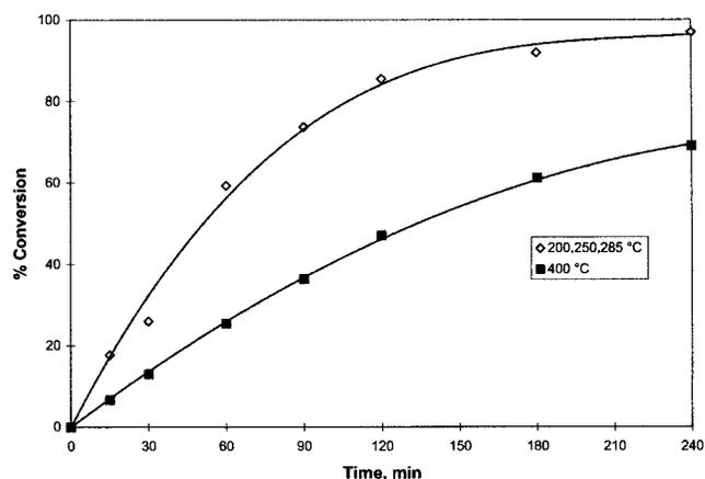
**Figure 2.** Effect of calcination temperature on benzene alkylation with 1-dodecene. C<sub>12</sub>:C<sub>6</sub>H<sub>6</sub>, 1:10 mol; catalyst DTP/K-10, 0.05 g/mL; temperature, 150 °C; speed, 1000 rpm; reaction time, 4 h.
