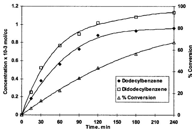
**Figure 6.** Effect of mol ratio on yields of mono- and dialkylated products in benzene alkylation with 1-dodecene. C<sub>12</sub>:C<sub>6</sub>H<sub>6</sub>, 2:1 mol; catalyst DTP/K-10, 0.05 g/mL, temperature, 150 °C; speed, 1000 rpm; reaction time, 4 h.
