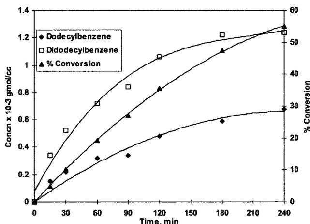
**Figure 7.** Effect of mol ratio on yields of mono- and dialkylated products in benzene alkylation with 1-dodecene. C<sub>12</sub>:C<sub>6</sub>H<sub>6</sub>, 5:1 mol; catalyst DTP/K-10, 0.05 g/mL, temperature, 150 °C; speed, 1000 rpm; reaction time, 4 h.
