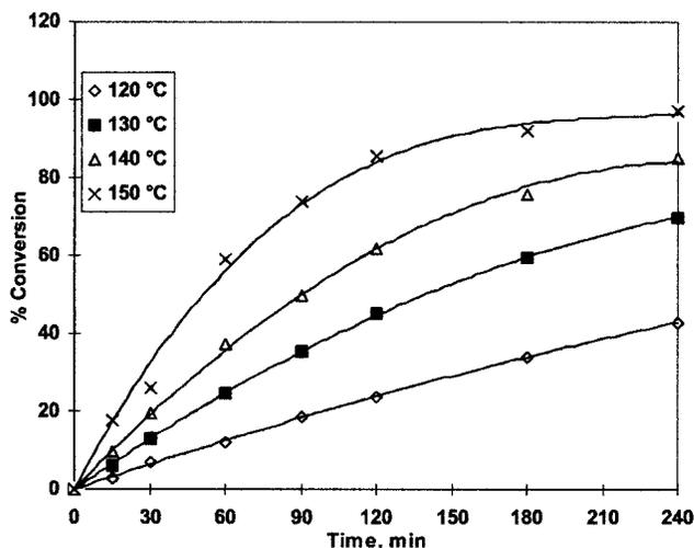
**Figure 10.** Effect of temperature on benzene alkylation with 1-dodecene.  $C_{12}:C_6H_6$ , 1:10 mol; catalyst DTP/K-10, 0.05 g/mL, temperature, 150 °C; speed, 1000 rpm; reaction time, 4 h.
