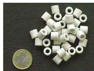
Figure 3. Megaporous glass Raschig rings.
