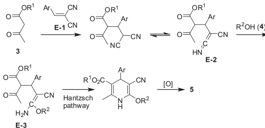
Scheme 2. Proposed pathway for the montmorillonite K-10 mediated synthesis of substituted cyano pyridines.
