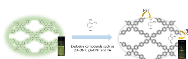
Scheme 2 Fluorescence quenching of TPE-CMP in the presence of nitroaromatic compounds via PET.
