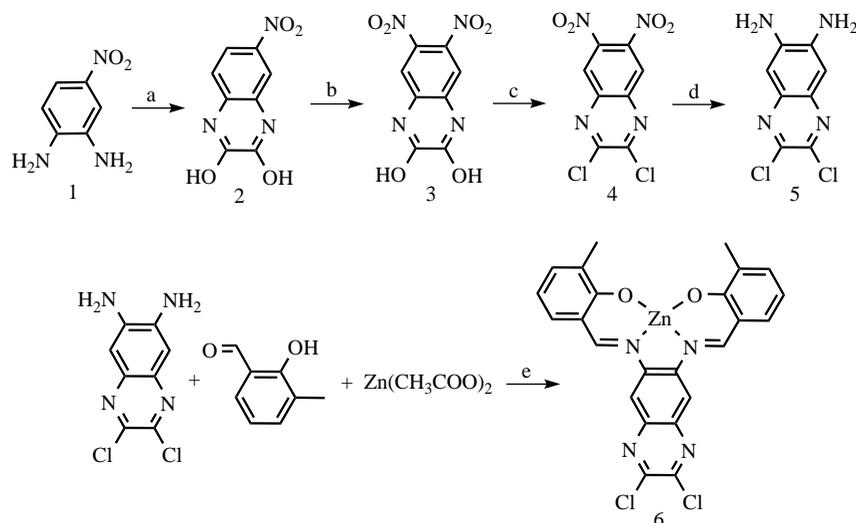
Scheme 1. Synthesis of Zn-salen quinoxaline. (a) Oxalic acid (1.5 equiv.), H<sub>2</sub>O, HCl, 115°C, 21 h. (b) KNO<sub>3</sub>, H<sub>2</sub>SO<sub>4</sub>, 0°C for 1 h and then at r.t. for 18 h. (c) POCl<sub>3</sub>, N-N-dimethylaniline, 110°C, 3 h. (d) SnCl<sub>2</sub>, HCl, EtOH, r.t., 1 h. (e) MeOH, r.t., 18 h.
