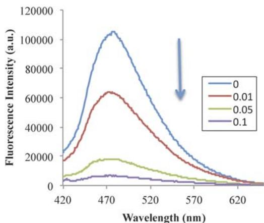
Figure 3. (Colour online) Fluorescence quenching of **Zn-Cav** by NT in acetonitrile. NT concentrations from the top spectrum to the bottom were 0, 0.010, 0.050 and 0.10 M.
